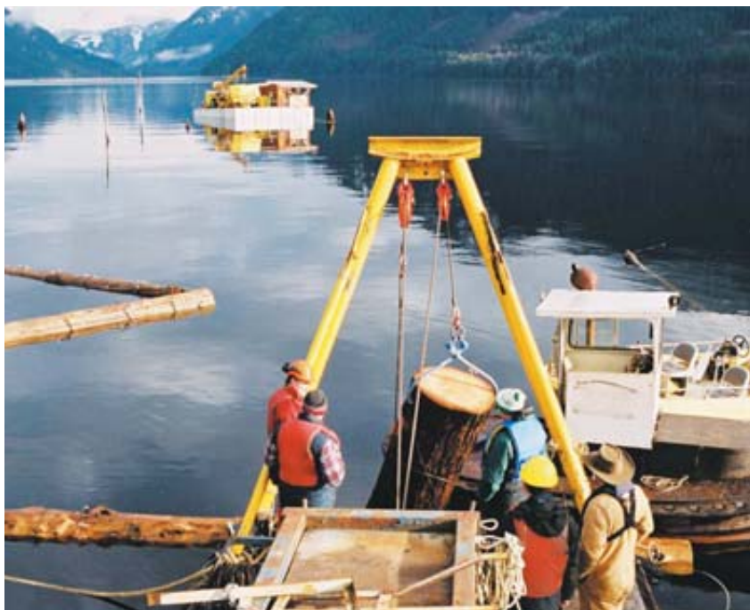
WATERLOGGED: Timber from a forest flooded under Lois Lake in British Columbia is lifted out of the water after being cut by Sawfish, a remotely operated vehicle seen in the background.
